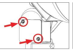
2. Remove wiring compartment access panel to knuckle wiring compartment by loosening two (2) screws using a 5/16" socket wrench.
