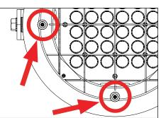
6. To relamp: remove faceplate and louver by loosening four (4) tamper resistant screws using a TORX T27 socket (1/4" bit). Relamp as needed, then reverse install.
