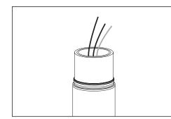
1. Pull branch circuit wiring needed, through pole tenon.
