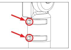
Fit fixture over pole on mounting plate and ensure it is completely seated. Secure fixture to pole by tightening two (2) 3/8"x16 stainless steel square screws using an adjustable crescent wrench.
