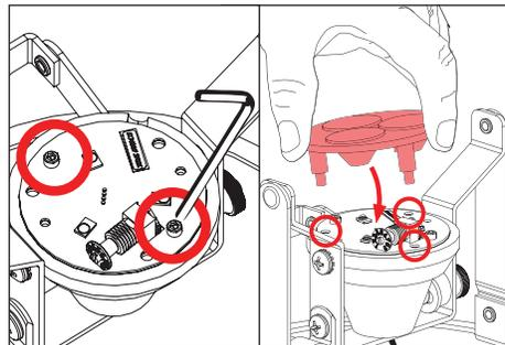
5. Secure LED board to heatsink by tightening two (2) #2-56 screws on LED board using a 5/64" allen wrench. Carefully snap optics back into tabs on LED board.
