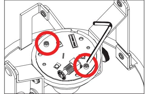
3. Use a 5/64" allen wrench to remove two (2) #2-56 screws on LED board. Grasp LED board gently and expose quick disconnect. Disengage LED board from driver assembly.
