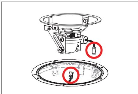
2. Connect OptiLock to secondary wiring via quick disconnect. Leads are labelled. Secondary wiring cable goes to splice location as per NEC. Make watertight connections from remote magnetic transformer to secondary cable wiring as per NEC. See wiring diagram.
