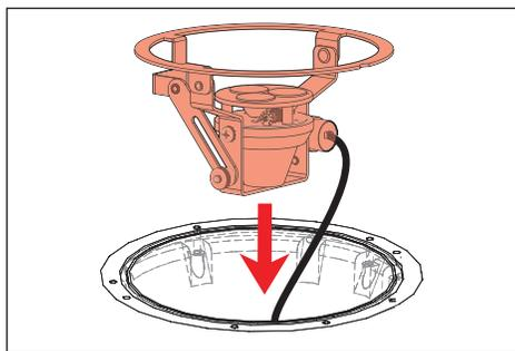
3. Place OptiLock in HP2 housing and align keyhole notch under one of two (2) #8 screw heads. Rotate horizontally to desired aiming position, then tighten two (2) #8 Phillips screws using Phillips screwdriver.
