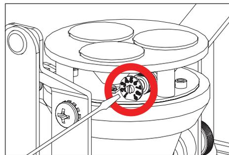
5. With flat head screw driver rotate Adjust-e-Lume dial to desired lumen output.
