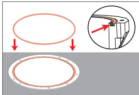
9. Remove any dirt or debris in o-ring groove near top of housing. Place o-ring inside of groove. Clean lens if needed.
