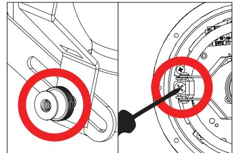
6. **If OptiLock Has Thumbscrew Aim:** Aim vertically by turning the thumbscrew on OptiLock assembly.
