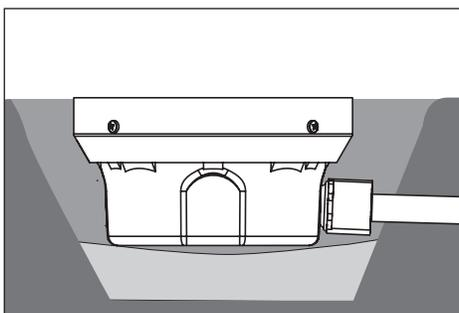
5. **For concrete installation:** Fill the hole around the fixture housing to 12" below the finished grade with clean fill dirt and tamp carefully to prevent settling of fixture. Pour concrete and finish as required flush with the top surface of the temporary cover.
