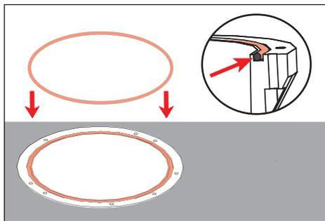
6. Remove any dirt or debris in o-ring groove near top of housing. Place o-ring inside of groove.
