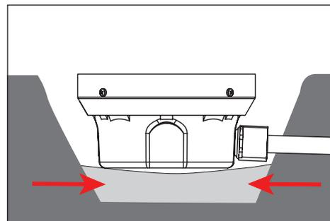
3. Per DIG-IT Guide, backfill the gap between the bottom of housing and bottom of hole with sand for drainage.
