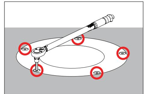
10. Install faceplate using a 1/8" allen wrench and hand-tighten the faceplate screws in a star pattern to 30 in-lbs. min.
