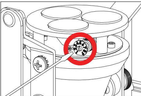
8. With flat head screw driver rotate Adjust-e-Lume® dial to desired lumen output.
