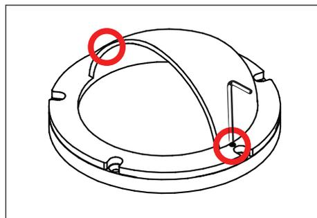
5. When set in final position, tighten two (2) #6-32 screws using a 7/64" allen wrench.
