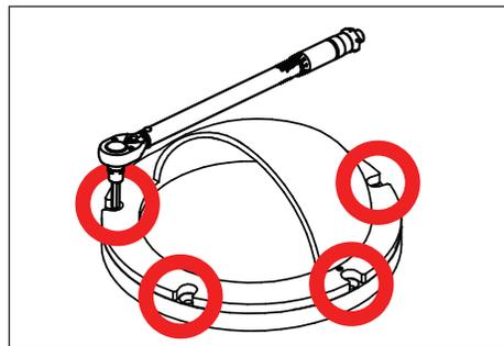
2. Install faceplate using a 1/8" allen wrench and hand-tighten the five (5) #10-24 faceplate screws in a star pattern to 30 in-lbs. min.
