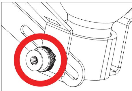
4. Aim vertically by turning the thumbscrew on OptiLock assembly.
