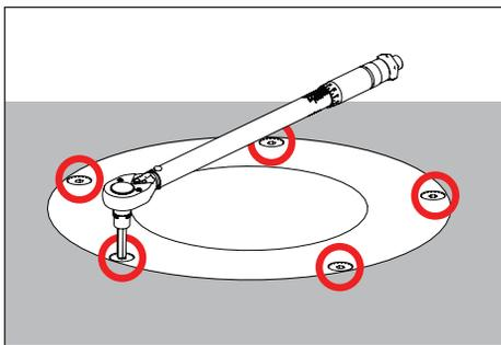
7. Install faceplate using a 1/8" allen wrench and hand-tighten the five (5) #10-24 faceplate screws in a star pattern to 30 in-lbs. min.
