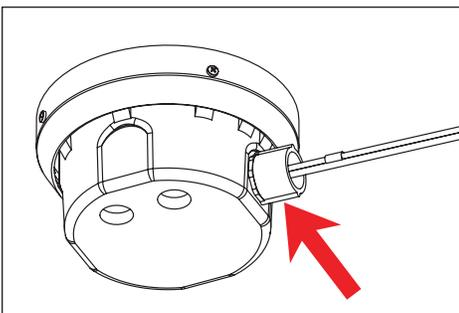
1. Secondary wiring is pre-wired with 5' leads. Pull 5' secondary leads from shallow HP2 housing through 3/4" conduit. Make watertight connections to secondary side of remote transformer using waterproof wire connectors in a waterproof splice compartment (not included) as per NEC.
