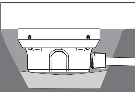
4. **For soil installation:** Fill and tamp soil to the appropriate height leaving room for sod, pavers, etc. to be level with the top of the faceplate.
