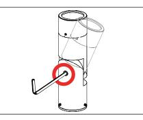
Insert wires and connectors into fixture base and attach to power pipe. To aim fixture, use a 3/16" allen wrench to slightly loosen ¼"-28 stainless steel black oxide socket head screw at the knuckle for vertical aiming purposes. Rotate fixture to aim to desired horizontal location.
