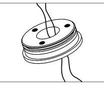
3. Pull wires from remote driver necessary for installation. Feed wiring through anchor base.
