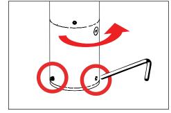
Use a 5/64" allen wrench to loosen (3) #8-32 stainless steel set screws on fixture base. Rotate fixture at base and aim fixture to desired horizontal location.
