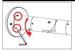
1. Use a 5/64" allen wrench to loosen three (3) #8-32 stainless steel set screws on fixture base. Rotate fixture at base and aim fixture to desired horizontal
