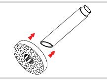
Slide optional stability flange onto power pipe. Use optional stability flange to aid in installation of power pipe.
