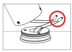
Make watertight connections from remote driver to fixture leads using waterproof wire connectors. See wiring diagram.
