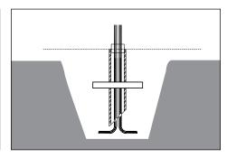
3. Pull wires from remote driver necessary for installation through power pipe. Allow for additional cable to make connections to fixture lead and future service. Place power pipe in hole.
