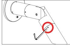
Use a 5/64" allen wrench to slightly loosen2. Remove optic by pulling gently and lift up. 1. three (3) #8-32 stainless steel set screws to remove cap.
