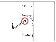
Tighten the three (3) #8-32 screws on base with appropriate tool for mounting method and stainless steel locking screw at the knuckle to secure all aiming positions.
