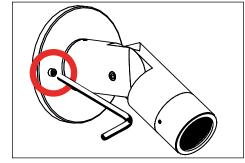
Use a 1/8" allen wrench to mount fixture with two (2) #10-24 hex screws to installed back box. Do not over tighten.
