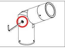
Tighten the three (3) #8-32 stainless steel set screws on anchor base and 1/4"-28 stainless steel locking screw at the knuckle to secure all aiming positions.
