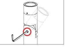
Use a 3/16" allen wrench to slightly loosen ¼"-28 stainless steel black oxide socket head cap screw at the knuckle for vertical aiming purposes.
