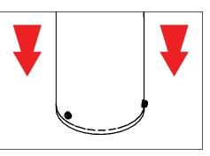
Place fixture onto mounted anchor base and press straight down until the two pieces are flush with each other.
