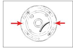
Install universal mounting ring (included with fixture) using appropriate mounting hardware. Align fixture mounting holes to final mounting position.
