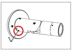
Tighten the three (3) #8-32 stainless steel set screws and 1/4"-28 stainless steel black oxide socket head cap screw at the knuckle to secure all aiming positions.
