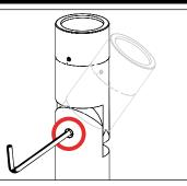
2. Use a 3/16" allen wrench to slightly loosen ¼"-28 stainless steel black oxide socket head cap screw at the knuckle for vertical aiming purposes.
