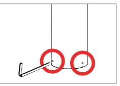
Tighten three (3) #8-32 stainless steel round head Phillips screws at base and 1/4"-28 stainless steel black oxide socket head screw at the knuckle to secure all aiming positions.
