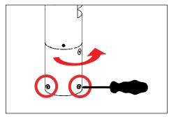
Use phillips screwdriver to loosen three (3) #8-32 stainless steel round head phillips screws at base. Rotate fixture at base and aim fixture to desired horizontal location.
