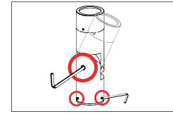
Use a 3/16" allen wrench to slightly loosen ¼"-28 stainless steel black oxide socket head cap screw at the knuckle for vertical aiming purposes. Rotate fixture at base and aim fixture to desired horizontal location.
