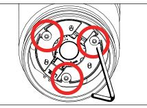
3. Use a .050" allen wrench to loosen three (3) set screws holding LED assembly. Gently lift LED assembly from fixture.
