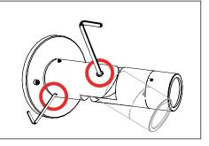
4. Use a 3/16" allen wrench to slightly loosen ¼"-28 stainless steel black oxide socket head cap screw at the knuckle for vertical aiming purposes. Use a 5/64" allen wrench to loosen the three (3) #8-32 stainless steel set screws. Rotate to aim fixture to desired horizontal location.
