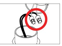
Make watertight connections from remote driver to fixture leads using waterproof wire connectors. See wiring diagram.
