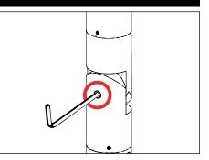
Tighten the three (3) #8-32 screws on base with appropriate tool for mounting method and stainless steel locking screw at the knuckle to secure all aiming positions.
