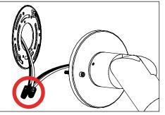
2. Pull wires from remote driver housing necessary for installation. Make watertight connections from remote driver housing to fixture leads using waterproof wire connectors. **See wiring diagram.**
