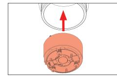
4. Install new LED assembly. Assembly can only connect in one direction. Secure set screws using a .050" allen wrench.
