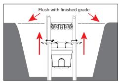
Raise housing on EMT so housing is flush with finished grade. Use a level to aid in housing installation.
