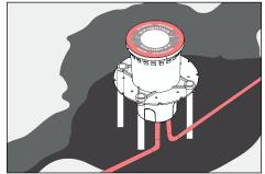
Pull primary branch circuit wiring into junction box.
