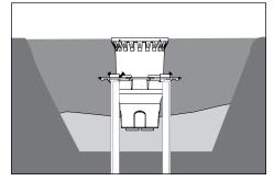
6. For concrete installation: Fill the hole around the fixture housing to 12" below the finished grade with clean fill dirt and tamp carefully to prevent settling of fixture. Pour concrete and finish as required flush with the top surface of the temporary cover.
