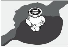
Place housing in hole. Align junction box in the path of the conduit trench.
