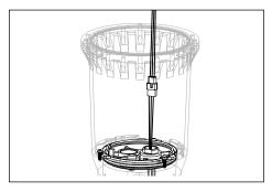
Connect optical assembly and faceplate to Patented HydroLock Barrier Plate with quick disconnect.
