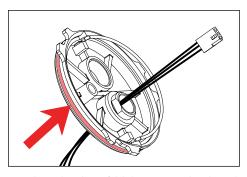
Wipe o-ring clean of debris on Patented HydroLock Barrier Plate. Install Patented HydroLock Barrier Plate by aligning keyholes with dometopped fasteners at the bottom of the housing and while grasping handle; push down on Patented HydroLock Barrier Plate until firmly seated.
