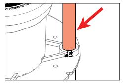
Insert four (4) pieces of ½" EMT conduit through the stability flange. Hammer into substrate until secure.
