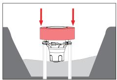
For soil installation: Fill and tamp soil to the appropriate height leaving room for sod, pavers, etc. to be level with the top of the temporary cover.
