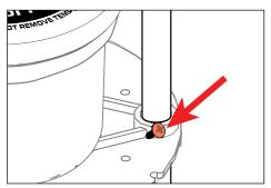
When housing is level, tighten screws on stability flange to secure housing to EMT. Remove excess EMT as needed.
