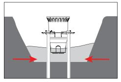
Per DIG-IT Guide, backfill the gap between the bottom of housing and bottom of hole with sand for drainage.
