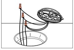
Make watertight connections using waterproof wire connectors (included) to leads on the bottom of Patented HydroLock Barrier Plate Assembly.
