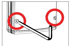
1. Loosen six (6) #10-24 captive screws using a 1/8" allen wrench to remove faceplate of UPM housing.
