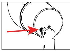
Press patented Anti-Condensation Valve (ACV) to release vacuum created inside the fixture during normal use. The valve is spring-loaded, by depressing it, air is allowed to re-enter the chamber and the pressure is then equalized. When the air-pressure equalizes the cap will release from body to allow service.
