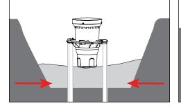
Per DIG-IT Guide, backfill the gap between the bottom of housing and bottom of hole with sand for drainage.
