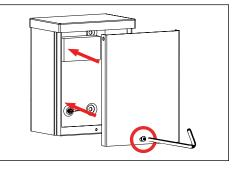
8. Re-attach cover. Tighten cover screw.
