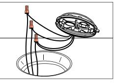
Make watertight connections using waterproof wire connectors (included) to leads on the bottom of Patented HydroLock Barrier Plate Assembly. See wiring diagram.
