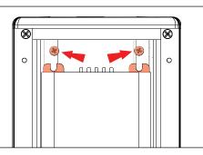
9. Remove two (2) #8-32 screws in UPM housing using Phillips screwdriver.
