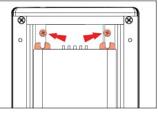
9. Remove two (2) #8-32 screws in UPM housing using phillips screwdriver.
