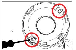
Use small phillips screwdriver to remove two (2) #4-40 fasteners on optic holder, then remove.
