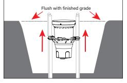
Raise housing on EMT so housing is flush with finished grade. Use a level to aid in housing installation.
