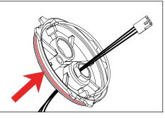
3. Wipe inside of housing where HydroLock plate will sit clean of debris before inserting patented HydroLock plate on to junction box. Align HydroLock plate with pins in housing and seat it firmly in place.
