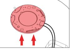
5. Carefully remove LED module from heatsink.
