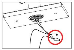
3. Make connections from remote power supply to fixture leads using proper wire connectors. **See wiring diagram.**
