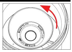
Remove optic by turning to the left to unlock optic from optic holder tabs, and lift up.
