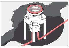
6. Pull primary branch circuit wiring into junction box.
