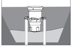
For concrete installation: Fill the hole around the fixture housing to 12" below the finished grade with clean fill dirt and tamp carefully to prevent settling of fixture. Pour concrete and finish as required flush with the top surface of the temporary cover.
