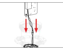
Connect the faceplate with the driver assembly to installed HydroLock with factory wired quick connectors. Lower faceplate assembly into housing.
