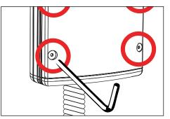
Make sure UPM housing gasket is free of any dirt or debris. Attach the faceplate by tightening the six (6) #10-24 captive screws evenly using a 1/8" allen wrench.
