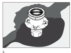
. Place housing in hole. Align junction box in the path of the conduit trench.
