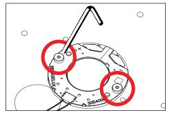
Spread thin, even layer of thermal paste on back of new LED module. Place new LED module onto heatsink, lining up module with holes for screws. Tighten two (2) #4-40 screws using a .050" allen wrench to secure LED module to heatsink.
