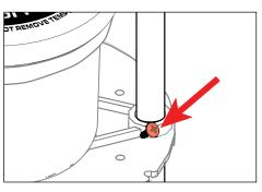
When housing is level, tighten screws on stability flange to secure housing to EMT. Remove excess EMT as needed.
