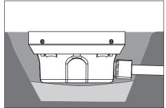
For concrete installation: Fill the hole around the fixture housing to 12" below the finished grade with clean fill dirt and tamp carefully to prevent settling of fixture. Pour concrete and finish as required flush with the top surface of the temporary cover.
