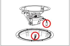
Connect OptiLock to secondary wiring via quick disconnect. Leads are labelled. Secondary wiring cable goes to splice location as per NEC. Make watertight connections from remote magnetic transformer to secondary cable wiring as per NEC. See wiring diagram.
