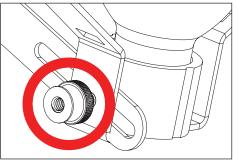
Aim vertically by turning the thumbscrew on 5. OptiLock assembly.
