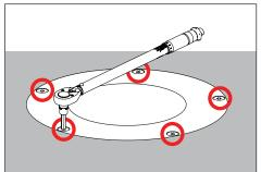
Install faceplate using a 1/8" allen wrench and hand-tighten the five (5) #10-24 faceplate screws in a star pattern to 30 in-lbs. min.
