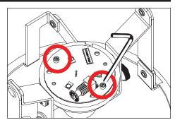
Use a 5/64" allen wrench to remove two (2) #2-56 screws on LED board. Grasp LED board gently and expose quick disconnect. Disengage LED board from driver assembly.
