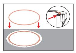
Remove any dirt or debris in o-ring groove near top of housing. Place o-ring inside of groove.
