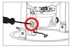
4. Use Phillips screwdriver to loosen #8-32 Phillips screw on driver bracket on OptiLock. Disconnect driver from fixture via quick disconnect. Replace old driver. Place new driver in bracket, then tighten #8-32 Phillips screw to secure new driver to OptiLock. Reconnect new replacement driver to fixture and to LED board via quick disconnects.
