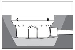
For soil installation: Fill and tamp soil to the appropriate height leaving room for sod, pavers, etc. to be level with the top of the faceplate.
