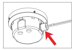
Secondary wiring is pre-wired with 5' leads. Pull 5' secondary leads from shallow HP2 housing though 3/4" conduit. Make watertight connections to secondary side of remote transformer using waterproof wire connectors in a waterproof splice compartment (not included) as per NEC.
