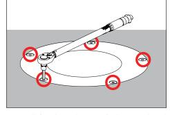
Install faceplate using a 1/8" allen wrench and hand-tighten the faceplate screws in a star pattern to 30 in-lbs. min.
