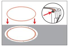
Remove any dirt or debris in o-ring groove near top of housing. Place o-ring inside of groove. Clean lens if needed.
