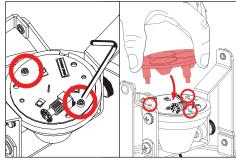
Secure LED board to heatsink by tightening two (2) #2-56 screws on LED board using a 5/64" allen wrench. Carefully snap optics back into tabs on LED hoard.
