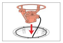
3. Place OptiLock in HP2 housing and align keyhole notch under one of two (2) #8 screw heads. Rotate horizontally to desired aiming position, then tighten two (2) #8 Phillips screws using Phillips screwdriver.
