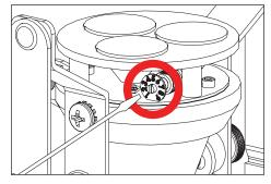
With flat head screw driver rotate Adjust-e-Lume® dial to desired lumen output.
