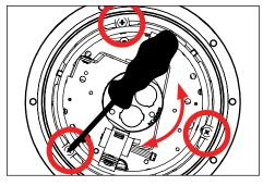
Place OptiLock in CO2 housing and align keyhole notch under one of three (3) #8 screw heads. Rotate horizontally to desired aiming position, then tighten two (2) #8 phillips screws using phillips screwdriver.
