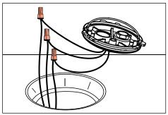
Make watertight connections using waterproof wire connectors (included) to leads on the bottom of Patented HydroLock Barrier Plate Assembly. See wiring diagram.
