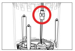
Connect OptiLock assembly to Patented HydroLock Barrier plate with quick disconnect.
