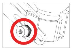
. Aim vertically by turning the thumbscrew on OptiLock assembly.
