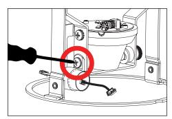
4. Use phillips screwdriver to loosen #8-32 phillips screw on driver bracket on OptiLock. Disconnect driver from fixture via quick disconnect. Replace old driver. Place new driver in bracket, then tighten #8-32 phillips screw to secure new driver to OptiLock. Reconnect new replacement driver to fixture and to LED board via quick disconnects.
