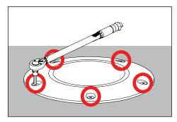
Install faceplate using a 1/8" allen wrench and hand-tighten the faceplate screws in a star pattern to 30 in-lhs, min.
