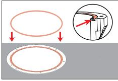
8. Remove any dirt or debris in o-ring groove near top of housing. Place o-ring inside of groove.
