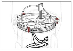
4. Turn HydroLock Barrier Plate clockwise 1/4" to lock.
