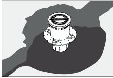
Place housing in hole. Align junction box in the path of the conduit trench.
