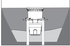
9. For concrete installation: Fill the hole around the fixture housing to 12" below the finished grade with clean fill dirt and tamp carefully to prevent settling of fixture. Pour concrete and finish as required flush with the top surface of the temporary cover.
