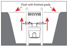
4. Raise housing on EMT so housing is flush with finished grade. Use a level to aid in housing
