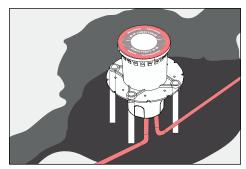
6. Pull primary branch circuit wiring into junction box.
