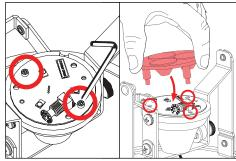
Secure LED board to heatsink by tightening two (2) #2-56 screws on LED board using a 5/64" allen wrench. Carefully snap optics back into tabs on LED board.
