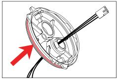
Wipe inside of housing where HydroLock plate will sit clean of debris before inserting patented HydroLock plate on to junction box. Align HydroLock plate with pins in housing and seat it firmly in place.
