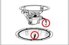
Connect OptiLock to secondary wiring via quick disconnect. Leads are labelled. Secondary wiring cable goes to splice location as per NEC. Make watertight connections from remote magnetic transformer to secondary cable wiring as per NEC. See wiring diagram.
