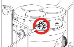
With flat head screw driver rotate Adjust-e-Lume dial to desired lumen output.
