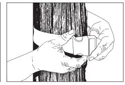
Use adjustable strap provided to attach UPM housing to tree. Tighten by pulling on the adjustable strap until secure.
