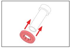
3. Slide stability flange onto housing.
