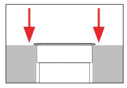
Place housing into hole. Surface mount collar should 3. rest on finished surface grade.
