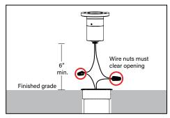
Access remote wiring inside housing. Make watertight connections using waterproof wire connectors. Wire connectors must clear opening. Insert fixture, wiring and connections into housing. See wiring diagram.
