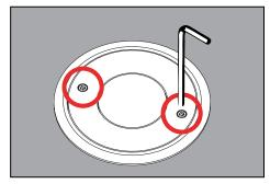
Mount faceplate to collar using two (2) #8-32 flat head screws (included) with a 9/64" allen wrench. Do not overtighten.
