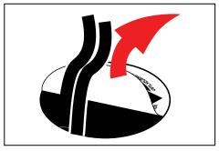
Remove temporary cover and pull out remote wiring.
