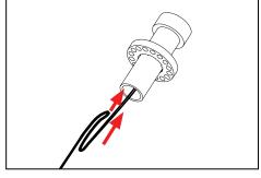
Loop minimum of 6" of low voltage wire inside housing to allow for fixture service. Place fixture in
