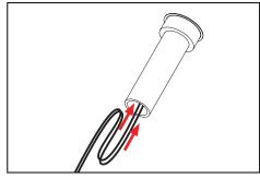
Loop minimum of 6" of wiring inside housing to allow for fixture service.
