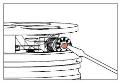
With flat head screw driver rotate dial to desired lumen output. Replace fixture in mounting collar.
