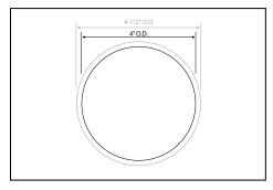
Drill 4" diameter hole into mounting surface at uplight 2. installation location as per lighting plan.
