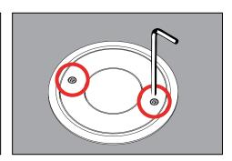
9. Mount faceplate to collar using two (2) #8-32 flat head screws (included) with a 9/64" allen wrench.
