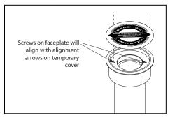
Align holes to final installation orientation. Arrows on temporary cover point towards screw location on faceplate for alignment purposes.
