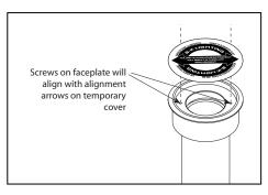
Orient the arrows on the temporary cover to the desired position of the final faceplate screw placement.
