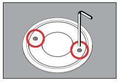
Remove faceplate from collar using two (2) #8-32 flat head screws (included) with a 9/64" allen wrench.
