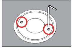
11. Mount faceplate to collar using two (2) #8-32 flat head screws (included) with a 9/64" allen wrench.
