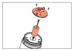
Reverse install LED board and driver by carefully engaging quick disconnects and inserting into fixture body. Secure LED board in place with stainless steel screws. Snap optics in place.
