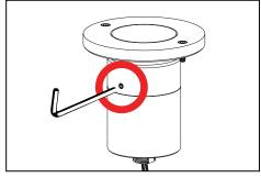
Loosen two (2) #8-32 screw with a 5/64" allen wrench to remove faceplate.
