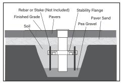
Per DIG-IT Guide, backfill the gap between the bottom of housing and bottom of hole with sand or pea gravel for drainage.
