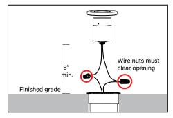
7. Access remote wiring inside housing. Make watertight connections using waterproof wire connectors. Wire nuts must clear opening. Insert fixture, wiring and connections into housing. See wiring diagram.
