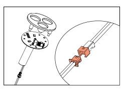
Disengage LED board and driver assembly. Replace with new board and driver assembly.
