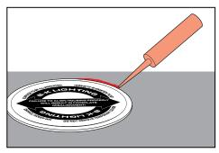
Use a silicone based sealant between fixture and 6. Remove temporary cover and pull out remote wiring. mounting surface.
