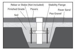
Fill with soil, then compress. Layer paver sand as required for paver installation, then install pavers. Pavers may need to be cut to fit around housing.
