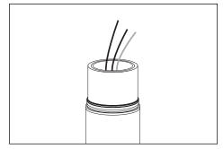
Pull branch circuit wiring needed, through pole tenon.
