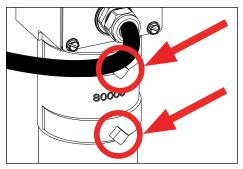
Slipfitter comes installed to fixture. Loosen two (2) 3/8-16 square head screws with adjustable wrench, then slide slipfitter with attached yoke and fixture to installed pole tenon on mounting plate until fully seated. Secure with two (2) 3/8-16 square head screws.
