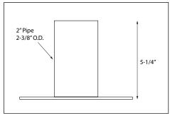
2. Pole in mounting plate has 2-3/8" O.D. and is 5-1/4"
