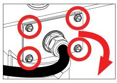
Place connections inside wiring compartment in slipfitter. Close panel to wiring compartment in slipfitter by tightening four (4) #10-24 hex washer heads using adjustable crescent wrench, 8mm socket wrench, or flat head screwdriver.
