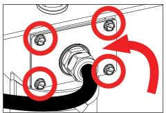
Open panel to wiring compartment in slipfitter by loosening four (4)#10-24 hex washer heads using adjustable crescent wrench, 8mm socket wrench, or flat head screwdriver.
