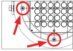
To relamp: remove faceplate and louver by loosening four (4) tamper resistant screws using a TORX T27 socket (1/4" bit). Relamp as needed, then reverse install.
