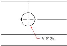
2. Clearance hole of yoke is 7/16" diameter.
