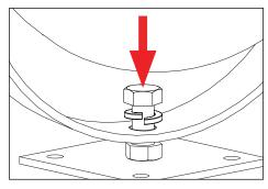
Line up fixture yoke to mounting plate and secure with 3/4"-10 bolt and locking washer (mounting hardware not included).
