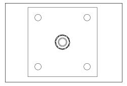
Install mounting plate in location as per lighting plan. Mounting plate has four (4) 9/16" dia. mounting holes 4-1/4" apart on center, square (mounting hardware not included).
