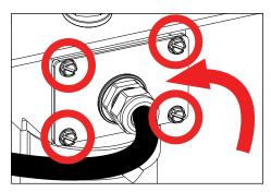
Open panel to wiring compartment in slipfitter by loosening four (4)#10-24 hex washer heads using adjustable crescent wrench, 8mm socket wrench, or flat head screwdriver.
