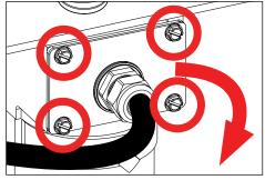
Place connections inside wiring compartment in slipfitter. Close panel to wiring compartment in slipfitter by tightening four (4)#10-24 hex washer heads using adjustable crescent wrench, 8mm socket wrench, or flat head screwdriver.
