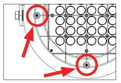
To relamp: remove faceplate and louver by loosening four (4) tamper resistant screws using a TORX T27 socket (1/4" bit). Relamp as needed, then reverse install.
