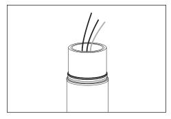
Pull branch circuit wiring needed, through 2" dia. pole tenon. Tenon has 2-3/8" O.D. (pole and tenon not included)
