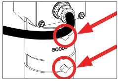
Slipfitter comes installed to fixture. Loosen two (2) 3/8-16 square head screws with adjustable wrench, then slide slipfitter with attached yoke and fixture to installed pole tenon. Secure with two (2) 3/8-16 square head screws
