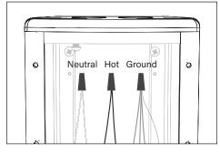
Use wire connectors (not included) to connect driver primary leads to branch circuit wires. Connect incoming ground to ground wire provided in UPM housing. See wiring diagram.
