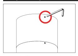
Loosen three (3) #10-32 set screws on base with a 3/32" allen wrench. Retain screws in fixture. Gently slide down fixture from mounting base to access ACV™ valve. Do not pull on install tether or leads.
