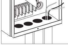
5. Pull branch circuit wiring necessary for installation.
