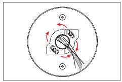
If UPM housing is not level, remove UPM housing; loosen but DO NOT REMOVE two (2) #8-32 screws with a 9/64" allen wrench on CamLock™ assembly. Adjust CamLock™ assembly up to 30° as needed to level. Tighten the screws and reattach UPM housing.
