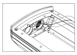
Pull branch circuit wiring and incoming dimming control wiring necessary for installation.
