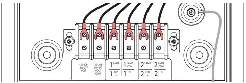
Terminal Block Wiring - Connect branch circuit to terminal block. Connect incoming ground to ground wire provided on NEMA 3R housing. Connect secondary lamp leads to terminal block. See labels on terminal block for additional information.
