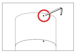
Place connections through wireway into junction box. Mount fixture over mounting plate, then secure with three (3) #10-32 screws using a 3/32" allen wrench. Do not overtighten.
