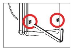
Make sure UPM housing gasket is free of any dirt or debris. Attach the faceplate by tightening the six (6) #10-24 captive screws evenly using a 1/8" allen wrench.
