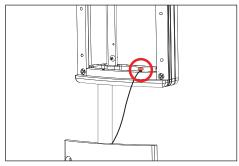
Attach tether wire under screw head at the base of the UPM housing and tighten. Slowly lower the faceplate until tether is taut.
