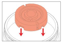
Place new LED module onto heatsink, lining up module with holes for screws.
