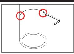
Loosen three (3) #10-32 stainless steel set screws on cap with a 5/32" allen wrench. Retain screws in
