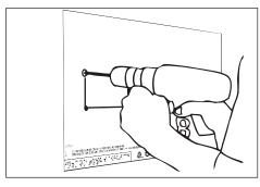
Drill holes into surface for ¼" fasteners on locations 3. illustrated on template.
