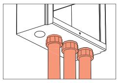
4. Connect conduit connector through female threaded conduit entry.
