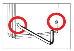
Loosen six (6) #10-24 captive screws using a 1/8" allen wrench and disconnect quick disconnect to remove faceplate of UPM housing.
