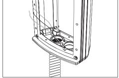
Pull branch circuit wiring and dimming control wiring necessary for installation.
