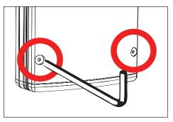
Loosen six (6) #10-24 captive screws using a 1/8" allen wrench to remove faceplate of UPM housing.
