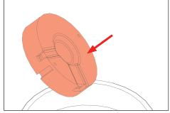
8. Spread thin, even layer of thermal paste on back of 9. new LED module.
