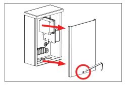
Remove cover by removing #10-24 cover screw using a 1/8" allen wrench.
