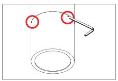
Place cap on fixture and tighten three (3) #10-32 set screws with a 3/32" allen wrench. Tighten screws to 1/2 in-lbs. Top of screws should sit flush with fixture cap.
