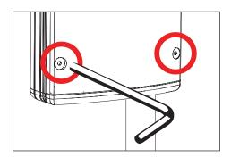
Make sure UPM housing gasket is free of any dirt or debris. Attach the faceplate by tightening the six (6) #10-24 captive screws evenly using a 1/8" allen
