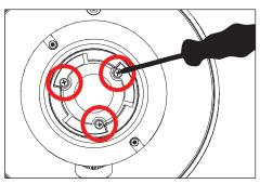
Loosen, then remove three (3) #2-28 screws from optic module using a phillips screwdriver. Remove optic holder from module.
