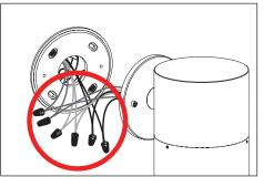
Make connections from remote driver and external dimming controls to fixture and module leads using proper wire connectors (not included). Number of wires and connections varies with wiring as per lighting plan. See wiring diagrams.
