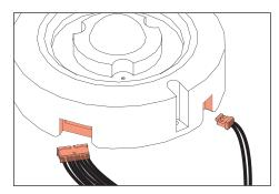
Carefully remove LED module from heatsink, then disconnect the quick disconnects for the wiring and the control wiring from the fixture to the LED module
