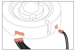
Connect new LED module to fixture via quick disconnects for wiring and for control wiring.
