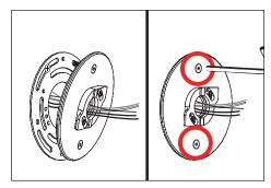
4. Feed branch circuit wiring and dimming control wiring through mounting plate with CamLock™ assembly. Attach mounting plate with supplied two (2) #10-24 stainless steel hex drive fasteners to universal ring using a 1/8" allen wrench.
