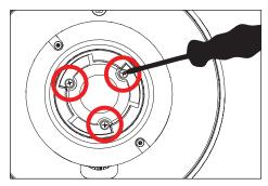
Place optic holder back on module. Tighten three
