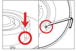
Loosen and remove two (2) #2-56 screws holding LED module to heatsink using a 0.050" allen
