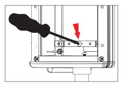
Remove the #8-32 screw in UPM housing using phillips screwdriver.
