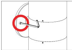
Place connections in back box, then mount fixture using two (2) #10-24 screws to installed back box using a 1/8" allen wrench. Seal building envelope as per NEC. Do not overtighten.
