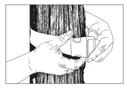
Use adjustable strap provided to attach UPM housing to tree. Tighten by pulling on the adjustable strap until secure.
