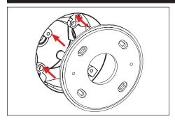
Install mounting ring (mounting ring included with fixture) using mounting hardware (not included) onto back box. Align fixture mounting holes to final mounting position.
