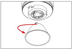
Gently twist optic to the left so optic tabs are clear of optic holder and carefully pull away.
