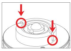
11. Secure LED module to heatsink with two (2) #2-56 screws using a 0.050" allen wrench.
