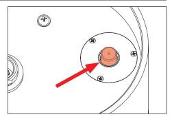
Press patented Anti-Condensation Valve (ACVTM) to release vacuum created inside the fixture during normal use. The valve is spring-loaded, by depressing it, air is allowed to re-enter the chamber and the pressure is then equalized. When the airpressure equalizes the cap will release from body to allow service.
