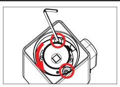
Rotate the two (2) 8-32 flat head cap screws using a 3/32" allen wrench clockwise until they bottom out into the heatsink then rotate the heatsink so they screws line up with the grooves. Remove the two (2) 8-32 flat head cap screws from the heatsink completely.
