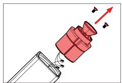
3. Disengage LED board and driver assembly.
