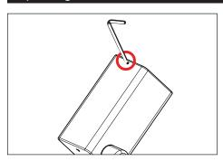
1. Use a 1/16" allen wrench to loosen #6-32 stainless set screw and remove cap.
