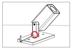
Use a 5/64" allen wrench to slightly loosen two (2) #8-32 stainless steel set screws on the stem for 360° aiming purpose.
