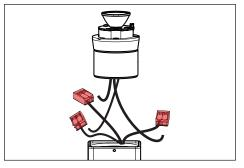
4. Disconnect driver assembly from fixture body.
