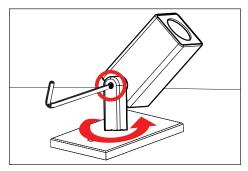
Use a 5/32" allen wrench to slightly loosen #10-32 stainless steel black oxide socket head cap screw at the knuckle for aiming purposes. Tighten to secure desired location.
