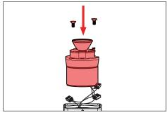
5. Connect new driver assembly to fixture leads. Place connections inside body cavity, reinsert new heatsink assy back into body. Reinstall two (2) 8-32 flat head cap screws completely onto the heatsink until screws catch under the groove on the body. Rotate the two (2) 8-32 flat head cap screws counterclockwise until they are snug against the top of the groove.
