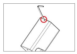
Place cap on fixture and tighten set screw. Tighten screw to 1/2 inch pounds. Top of screw should sit flush with fixture body.
