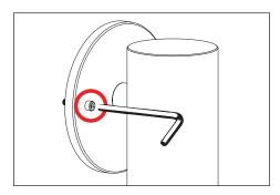
Mount fixture using two (2) #10-24 hex screws to installed back box. Seal building envelope as per NEC. Do not overtighten.
