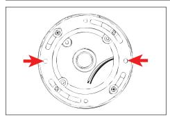
Install universal mounting ring (supplied with fixture) using #10-24 screws onto back box. Align fixture mounting holes to final mounting position.
