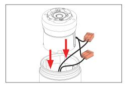
Connect new driver assembly to fixture leads. Place connections inside body cavity, then slide down fixture body along guides.
