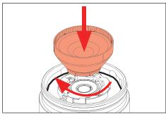
10. Twist to reinstall optic onto optic holder.
