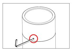
Install cap by tightening three (3) #8-32 set screws with a 5/64" allen wrench. **Do not over tighten.** Cap should be able to rotate without force.
