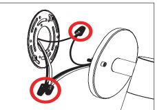
Make watertight connections from remote driver to fixture source leads using waterproof wire connectors (not included). See wiring diagram.
