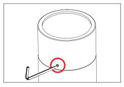
Loosen three (3) #8-32 set screws with a 5/64" 2. Twist and pull away optic. allen wrench on cap, then remove cap.
