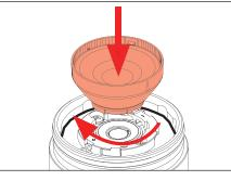
10. Twist to reinstall optic onto optic holder.
