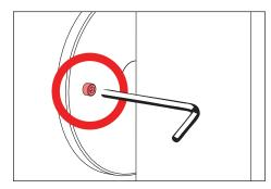
3. Mount fixture using two (2) #10-24 hex screws to installed back box. Seal building envelope as per NEC. Do not overtighten.
