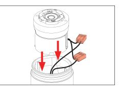
8. Connect new driver assembly to fixture leads. Place connections inside body cavity, then slide down fixture body along guides.
