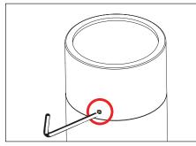
1. Loosen three (3) #8-32 set screws with a 5/64" 2. Twist and pull away optic. allen wrench on cap, then remove cap.
