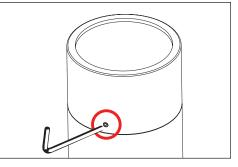
Install cap by tightening three (3) #8-32 set screws with a 5/64" allen wrench. **Do not over tighten.** 11. Cap should be able to rotate without force.
