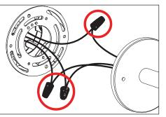
2. Make watertight connections from remote driver to fixture source leads using waterproof wire connectors (not included). See wiring diagram.
