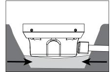
Per DIG-IT Guide, backfill the gap between the bottom of housing and bottom of hole with sand for drainage.
