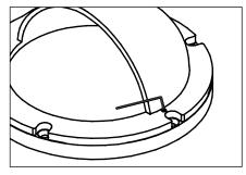
When set in final position, tighten two (2) #6-32 set screws using a 7/64" allen wrench.
