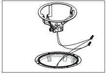
Make connections using silicone filled wire nuts (provided) from OptiLock to secondary wiring. See wiring diagram.
