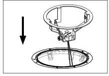
3. Place OptiLock in HP2 housing and align keyhole notch under one of three (3) #8 screw heads. Rotate horizontally to desired aiming position, then tighten two (2) #8 Phillips screws using Phillips screwdriver. Install proper MR16 halogen or PAR36/AR111 lamp according to instructions on Lamp Installation Or Re-Lamping page.
