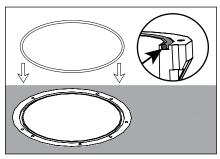
Remove any dirt or debris in o-ring groove near top of housing. Place o-ring inside of groove.
