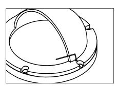
Using a 7/64" allen wrench, loosen the two (2) #6-32 set screws on the faceplate to allow accessory to rotate freely.
