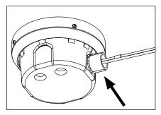
Secondary wiring is pre-wired with 5' leads. Pull 5' secondary leads from shallow HP2 housing though 3/4" conduit. Make watertight connections to secondary side of remote transformer using waterproof wire connectors in a waterproof splice compartment (not included) as per NEC.
