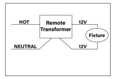
WIRING DIAGRAM FOR USE WITH:
