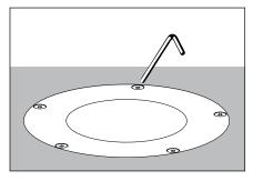
Install faceplate using a 1/8" allen wrench and hand-tighten the faceplate screws in a star pattern to 30 in-lbs. min.
