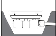
Place housing in excavated hole. Align power cord with leads in the path of the conduit trench(es).
