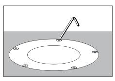
Remove faceplate using a 1/8" allen wrench. If there is an optional accessory holder, carefully squeeze tabs on sides and gently pull from slots on OptiLock.
