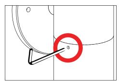
1. Loosen three (3) #8-32 X 1/8<sup>m</sup> stainless steel set screws with a 5/64" allen wrench on cap. Retain screws in cap.
