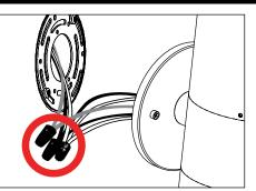
2. Make connections with branch circuit wiring to lamp leads using proper wire connectors (not included). Connect grounding wire to ground wire from fixture. See wiring diagram.
