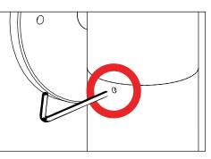
3. Replace cap on fixture and tighten three (3) #8-32 x 1/8" stainless steel set screws with a 5/64" allen wrench.
