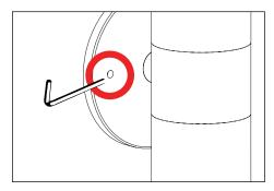
Mount fixture using two (2) #10-24 hex screws to installed back box using a 1/8" allen wrench. Seal building envelope as per NEC. Do not overtighten.
