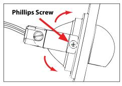
Loosen Phillips screws on adjustable lamp bracket and aim lamp to desired angle. When angle is set, tighten Phillips screw to lock in place.
