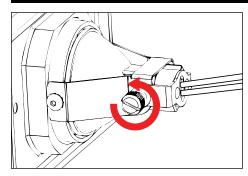
To install lamp (if needed), remove socket assembly from faceplate housing by loosening thumbscrew. Do not exceed wattage on label.
