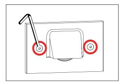
Mount faceplate using two (2) #10-24 screws with a 1/8" allen wrench. Tighten to compress gasket. Do not over tighten.
