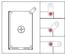
To prepare MB2 for mounting, align mounting brackets on back of box. Brackets can be aligned to vertical, horizontal or 45° orientation. Secure with mounting screw using screwdriver.
