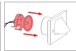
3. Re-insert socket assembly into faceplate.
