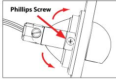
Loosen phillip screws on adjustable lamp bracket and aim lamp to desired angle. When angle is set, tighten phillip screw to lock in place.
