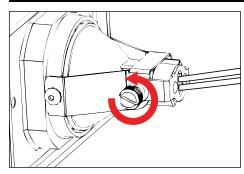
To install lamp (if needed), remove socket assembly from faceplate housing by loosening thumbscrew.
