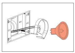
Remove socket assembly from faceplate housing. Install lamp if needed. Do not exceed wattage on label.
