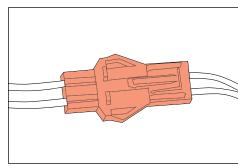
Connect quick disconnect from thermal protector to lamp leads.
