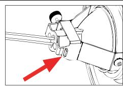
Insert tab from socket into notch on adjustable lamp bracket, then tighten thumbscrew.
