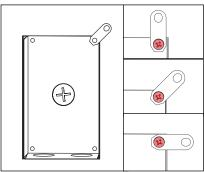
To prepare MB2 for mounting, align mounting brackets on back of box. Brackets can be aligned to vertical, horizontal or 45° orientation. Secure with mounting screw using screwdriver.
