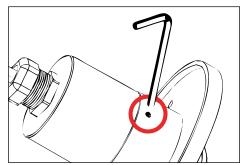
Re-attach faceplate to core drill body and tighten set screw. Do not over tighten!
