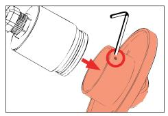
1. Loosen 5/64" set screw to remove faceplate.
