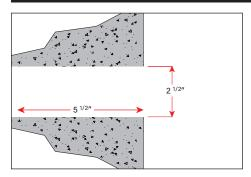
Core drill a 2 1/2" hole 5 1/2" deep into a noncombustible material.
