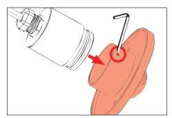
1. Loosen 5/64" set screw to remove faceplate.
