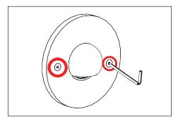
Install fixture into core drilled hole and mount with two (2) #10 fasteners as required (mounting screws not included). Length and type of mounting screws will vary with construction material.
