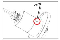
Re-attach faceplate to core drill body and tighten set screw.
