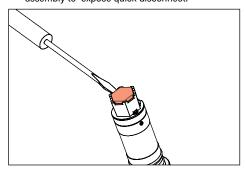
Use small flat head screw driver to remove lens from optic holder on the LED. Snap new optic in place. Replace cap on fixture and tighten set screw.
