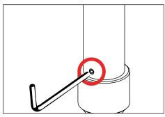
Use a 5/64" allen wrench to loosen #8-32 stainless steel set screw and remove cap.
