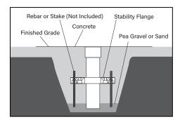
Fill the hole around the fixture housing to 12" below the finished grade with clean fill dirt and tamp carefully to prevent settling of fixture. Pour concrete and finish as required flush with mounting collar.
