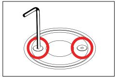
11. Mount faceplate to collar using two (2) #6-32 screws (included) with a 5/64" allen wrench.
