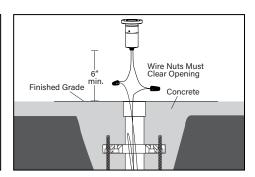
Access low voltage wire inside power pipe. Make two watertight connections using waterproof wire connectors. Wire nuts must clear opening. Insert fixture and low voltage wire into housing. See wiring diagram.
