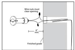
Pull low voltage wire through flush mount collar and make two watertight connections using waterproof wire connectors (not included). Insert wires and fixture back into hole. Wire connectors must clear opening. See wiring diagram.
