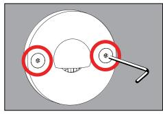
Mount faceplate to collar using two (2) #6-32 flat head cap screws with a 5/64" allen wrench.
