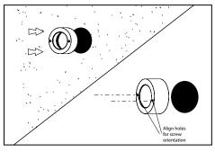
4. Fit surface mount collar into hole so it is flush with finished surface. Wipe off any excess adhesive.
