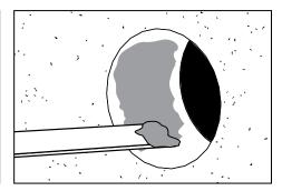
Use mixing stick to apply the epoxy to the interior of the hole as shown.
