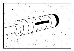
Core drill 1-3/4" dia. through hole into material for mounting collar minimum 4-1/2" deep. If wire way is needed, drill 1/2" dia. hole as necessary for 18-gauge 2-wire low voltage cable.
