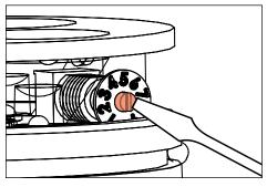
With flat head screw driver rotate dial to desired lumen output.
