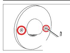
Remove fixture by loosening Gently pull away faceplate aw fixture body.
