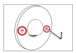
Install fixture into core drilled hole and mount with two (2) #10 fasteners as required (hardware not included). Length and type of mounting screws will vary with construction material. Tighten evenly to compress gasket. Do not over tighten.
