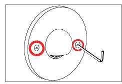
. Mount faceplate using two (2) #10 fasteners as required. Length and type of mounting screws will vary with construction material. Tighten evenly to compress gasket. **Do not over tighten.**
