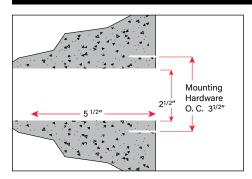
Core drill a 2 1/2" hole 5 1/2" deep into mounting structure. Leave sufficient material between core drill hole and anchor mount.
