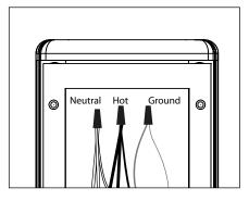
Use wire connectors (By Others) to connect both 7. transformers primary leads to branch circuit wires. Connect incoming ground to ground wire provided in UPM housing. See wiring diagram.
