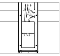
Remove the backing from adhesive tape on transformers, place in bottom of UPM body void of any wiring and press firmly for five seconds to ensure good contact.
