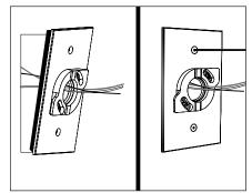
Feed branch circuit wiring and lamp leads to remote mounted fixture through mounting plate with CamLock<sup>™</sup> assembly. Attach mounting plate with supplied (2) #6-32 stainless steel hex drive fasteners to recessed junction box using a 5/64" allen wrench.
