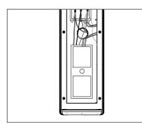
Remove the backing from adhesive tape on transformers, place in bottom of UPM housing void of any wiring and press firmly for five seconds to ensure good contact.
