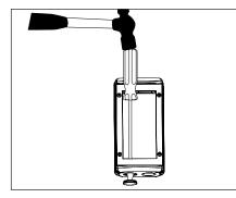
Remove Patented Knockout(s) as necessary from the inside of the UPM housing for branch circuit wiring and lamp leads to remote mounted fixture. Leave remaining unused knockouts in place to maintain seal.
