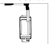
Remove Patented Knockout(s) as necessary from the inside of the UPM housing for branch circuit wiring and lamp leads to remote mounted fixture. Leave remaining unused knockouts in place to maintain seal.
