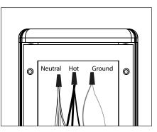
Use wire connectors (By Others) to connect both transformers primary leads to branch circuit wires. Connect incoming ground to ground wire provided in UPM housing. See wiring diagram.
