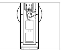
10. Remove the backing from adhesive tape on transformers, place in bottom of UPM housing void of any wiring and press firmly for five seconds to ensure good contact.
