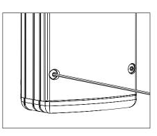
Make sure UPM body gasket is free of any dirt or debris. Attach the faceplate by tightening the (4) #6-32 captive screws evenly to 6-9 in/lbs using a 5/64" allen wrench.
