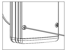
Make sure UPM body gasket is free of any dirt or debris. Attach the faceplate by tightening the (4) #6-32 captive screws evenly to 6-9 in/lbs using a 5/64" allen wrench.
