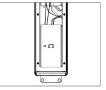
Remove the backing from adhesive tape on transformers, place in bottom of UPM housing 9. void of any wiring and press firmly for five seconds to ensure good contact.
