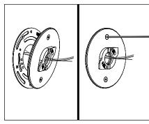
4. Feed branch circuit wiring and lamp leads to remote mounted fixture through mounting plate with CamLock™ assembly. Attach mounting plate with supplied (2) #10-24 stainless steel hex drive fasteners to universal ring using 1/8" allen wrench.
