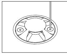
10. Mount faceplate to collar using (2) #6-32x5/8" flat head screws (provided) with a 5/64" Allen wrench.
