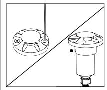
Loosen #8-32 set screw on faceplate assembly using a 5/64" Allen wrench and remove. Loosen set screw on collar and remove.
