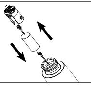
Pull the heat sink from the body to expose the LED board and Driver components. Utilize quick disconnects to change modular LED and driver components. Re-install the heat sink into body.
