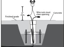
Access low voltage wire inside Power Pipe<sup>™</sup>. Make two watertight connections using waterproof wire connectors (By Others). Wire nuts must clear opening. Insert fixture and low voltage wire into Power Pipe<sup>™</sup>.
