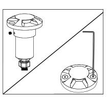
3. Replace faceplate assembly and tighten set screw. Re-Install fixture.
