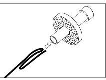
Loop minimum of 6" of low voltage wire inside Power Pipe™ to allow for fixture service.
