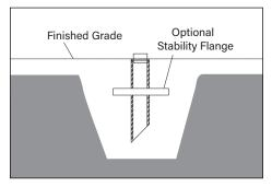
Excavate trench according to designed lighting plan. Dig hole a minimum of 24" deep and 10" wide to accommodate ower pipe at desired fixture locations.
