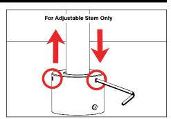
4. Slide stem up or down to desired height. Delrin bushing holds stem in position. Tighten three (3) #10 stainless steel set screws using a 3/32" allen wrench to lock mounting height in place. Unused stem length remains hidden inside power pipe to accommodate future landscape growth.
