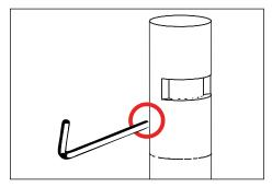
1. Loosen #8-32 stainless steel set screw on cap using a 2. 5/64" Allen wrench and remove.
