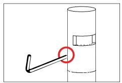
Place cap on fixture and tighten set screw. Tighten screw to 1/2 inch pounds. Top of screw should sit flush with fixture cap.
