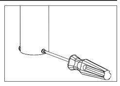
Insert wires, connectors and/or transformer into fixture base and attach to power pipe. Tighten three (3) #8-32 stainless steel round head phillips screws at base to secure.
