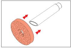
Slide optional stability flange onto power pipe. Use optional stability flange to aid in installation of power pipe.  Pull low voltage wiring from remote transformer to power pipe. Allow for additional cable to make connections to fixture lead and future service.
