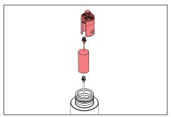
For BKSSL: Pull the heat sink from the body to expose the LED board and Driver components. Utilize quick disconnects to change modular LED and driver components. Re-install the heat sink into body.
