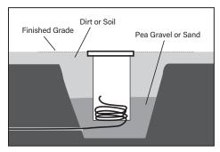
Align and orientate concrete pour collar on housing to illuminated object. Back fill with pea gravel or sand to allow sufficient drainage. Install housing flush at grade. See wiring diagram.
