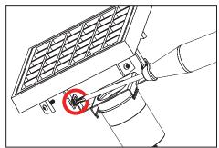
Loosen stainless steel phillips head cap screw on adjustable bracket, aim to desired location. Tighten to maintain aiming position.
