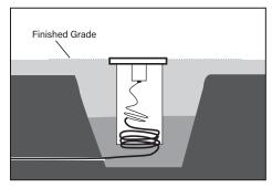
Attach faceplate to concrete pour collar with four (4) 1/4-20 screws using a 3/16" allen wrench.
