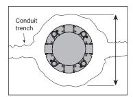
Excavate a hole to the necessary dimensions for fixture placement according to lighting plan.
