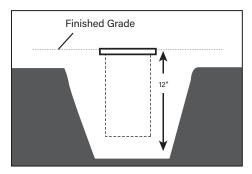
Excavate trench according to designed lighting plan 20" deep and 10" wide suitable for the 13" fixture housing.
