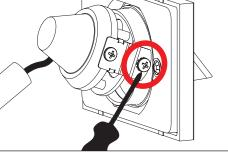
To aim, loosen the two (2) phillips screws attaching the adjustable bracket to the faceplate. Aim to desired position. Tighten two (2) phillips screws to 2. lock in place when desired angle is set.
