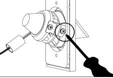
To aim adjustable bracket loosen the two (2) phillip 2. screws attaching the adjustable bracket to the faceplate. Aim to desired position. Tighten two (2) phillip screws to lock in place when desired angle is set.
