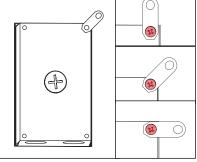
То prepare MB2 for mounting, align mounting brackets on back of box. Brackets can be aligned to vertical, horizontal or 45° orientation. Secure with mounting screw using screwdriver.
