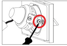
Attach bracket to faceplate by securing two (2) phillips screws. Aim to desired position. Tighten two (2) phillips screws to lock in place when desired angle is set.
