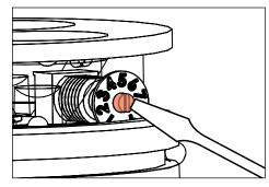
7. With flat head screw driver rotate dial to desired lumen output.
