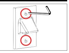
Mount faceplate using two (2) #10-24 screws with 1/8" allen wrench. Tighten evenly to compress 3. gasket. Do not over tighten.
