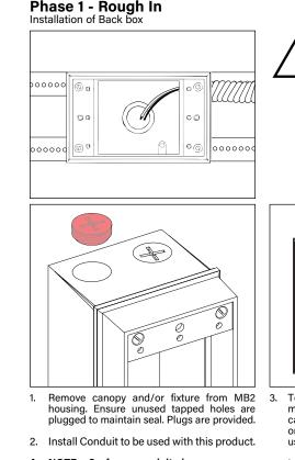
NOTE: Surface conduit is a common 凶 entrance for water if not properly sealed. Seal connector threads and conduit with a suitable sealant (teflon tape, adhesive, etc.). Sealing the conduit after knockouts are removed is required to maintain warranty.
