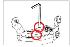
Use a 5/64" allen wrench to remove two (2) socket head cap screws on LED board, LED board and gently pull up to expose disconnect.
