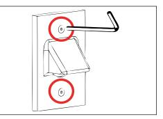
9. Mount faceplate using two (2) #10-24 screws with a 1/8" allen wrench. Tighten evenly to compress gasket. **Do not over tighten.**
