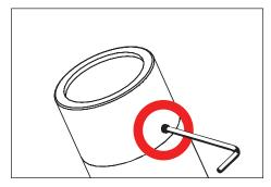
Place cap on fixture and tighten set screw. Tighten screw to 1/2 in-lbs. Top of screw should sit flush with fixture cap.
