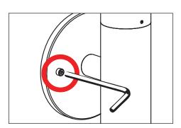
Using a 5/32" allen wrench mount fixture using two (2) #10-24 screws to installed back box. Seal building envelope as per NEC. Do not overtighten.
