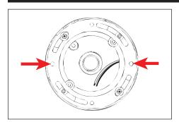
Install universal mounting ring (included with fixture) using #10-24 screws onto back box. Align fixture mounting holes to final mounting position. Universal mounting ring orientation determines fixture orientation.
