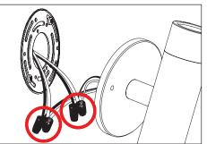
Make watertight connections from remote transformer to fixture leads using waterproof wire connectors. See wiring diagram.
