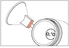
2. Firmly insert lamp pins into socket to make connection. Rocking motion may be required.
