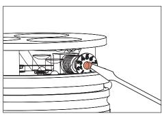
2. With flat head screw driver rotate dial to desired lumen output.
