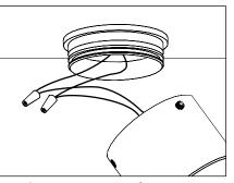
6. Make two connections from remote 12V transformer to fixture source leads using proper wire connectors (By Others). See wiring diagram.
