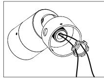
3. Mount knuckle onto canopy by securing 1/2" NPS stem with provided locknut.
