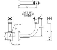
YWB - Yoke Mount (YM) with Wall Bracket
