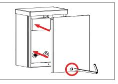
8. Re-attach cover. Tighten cover screw.
