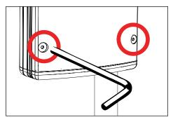
Slide driver feet under two screws in UPM housing and tighten screws using Phillips screwdriver.
