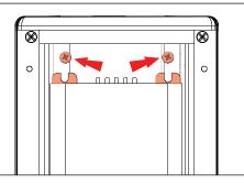
9. Remove two (2) #8-32 screws in UPM housing using Phillips screwdriver.
