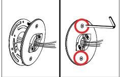
Feed branch circuit wiring and dimming control wiring through mounting plate with CamLock assembly. Attach mounting plate with included two (2) #10-24 stainless steel hex drive fasteners to universal ring using a 1/8" allen wrench.
