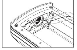
7. Pull branch circuit wiring and dimming control wiring necessary for installation.
