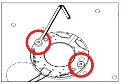
Spread thin, even layer of thermal paste on back of new LED module. Place new LED module onto heatsink, lining up module with holes for screws. Tighten two (2) #4-40 screws using a .050" allen wrench to secure LED module to heatsink.
