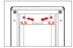
10. Remove two (2) #8-32 screws in UPM housing using Phillips screwdriver.
