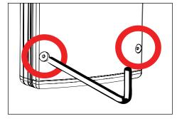
1. Loosen six (6) #10-24 captive screws using a 1/8" allen wrench to remove faceplate of UPM housing.
