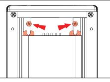
Remove two (2) #8-32 screws in UPM housing using phillips screwdriver.
