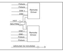
Use waterproof wire connectors (By Others) to connect driver primary leads to branch circuit wires. Connect incoming ground to ground wire
