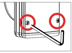
Make sure UPM housing gasket is free of any dirt or debris. Attach the faceplate by tightening the six (6) #10-24 captive screws evenly using a 1/8" allen wrench.
