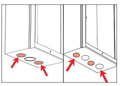
Remove knockout(s) with hammer as needed from the NEMA 3R housing. Leave remaining unused knockouts in place to maintain seal.
