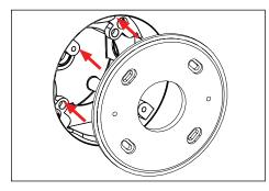
Install heavy duty mounting ring (mounting ring supplied with fixture) using mounting hardware (not included) onto back box. Align fixture mounting holes to final mounting position.
