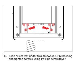
tighten to secure driver to UPM housing.
