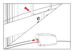
4. Thread safety cable through hole on the back of the UPM housing. Feed safety cable through opposing ends of the connector. Pull on wires to assure the connection is secure. Leave enough slack in safety cable for tree growth. Adjustments can be made by pressing release spring with a pin or a 3/64" allen tool.
