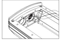
7. Pull branch circuit wiring and dimming control wiring necessary for installation.
