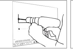
Drill holes into surface for ¼" fasteners on locations required for mounting via tabs.
