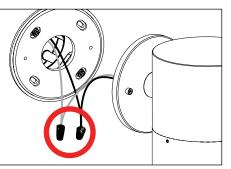
Make connections from remote driver and external dimming controls to fixture and module leads using proper wire connectors (not included). Number of wires and connections varies with wiring as per lighting plan. See wiring diagrams.
