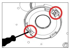
Unscrew #4-40 phillips fasteners on optic holder using phillips screwdriver. Grasp optic holder and gently pull upward to remove.
