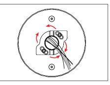
If UPM housing is not level, remove UPM housing; loosen but **DO NOT REMOVE** two (2) #8-32 screws with a 9/64" allen wrench on CamLock assembly. Adjust CamLock assembly up to 30° as needed to level. Tighten the screws and reattach UPM housing.
