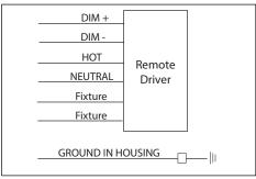
Use waterproof wire connectors to connect driver primary leads to branch circuit wires. Connect incoming ground to ground wire provided in UPM
