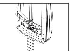
6. Pull branch circuit wiring and dimming control wiring necessary for installation.
