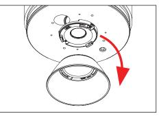
1. Loosen three (3) #10-32 stainless steel set screws on cap with a 5/32" allen wrench. Retain screws in cap.
