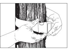
Use adjustable strap provided to attach UPM housing to tree. Tighten by pulling on the adjustable strap until secure.
