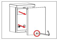
1. Remove cover by removing #10-24 cover screw using a 1/8" allen wrench.
