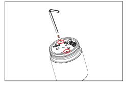
Use a 5/64" allen wrench to remove two (2) #2-56 socket head cap screws on LED board, grasp LED board and gently pull up to expose quick
