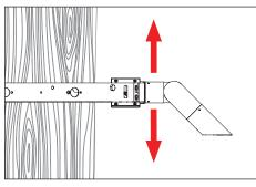
1. Place tree ring fixture around tree. Move fixture to desired height. Tighten the entire assembly to the tree with provided stand-offs.
