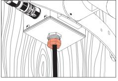
Bring line voltage cable from power line to main splice box location. Loosen cord grip on bottom of splice box, feed line voltage cable from power line through, then tighten cord grip to secure
