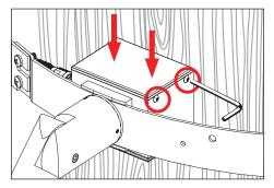
7. Replace top of driver housing with four (4) #8-32 screws with a 5/64" allen wrench.
