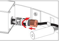
3. Connect secondary cable then twist to secure in place.
