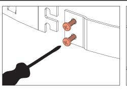
2. Secure by hooking end of strap over two (2) phillips screws. Secure by tightening two (2) phillips screws with phillips screwdriver.
