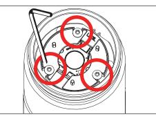
3. Use a 0.050" allen wrench to loosen three (3) set screws holding LED assembly. Gently lift LED assembly from fixture.
