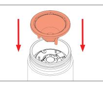
5. Replace optic by lining notches with optic holder, then pressing down gently until secured into place.
