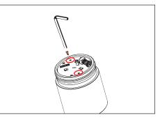
Use a 5/64" allen wrench to remove two (2) #2-56 socket head cap screws on LED board, grasp LED board and gently pull up to expose quick disconnect.
