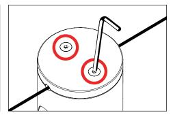
Install clamp to splice compartment to 1/4" O.D. aircraft cable with two (2) #10-24 cap screws using 3. a 1/8" allen wrench.
