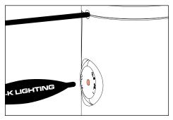
Pierce center of break-thru plug with ball point pen 5.
