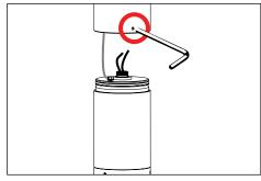
Use a 5/64" allen wrench to separate splice compartment and fixture body.
