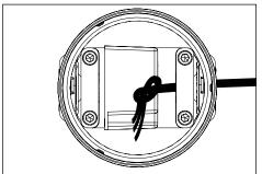
. Tie underwriter's knot in cable for additional strain relief between connections and clamp.
