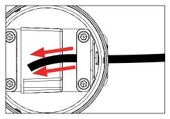
Thread incoming 3 wire ROUND jacketed line voltage cable through grommet, then through strain relief clamp.
