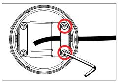
Secure strain relief clamp by tightening two (2) 3. #8-32 screws with a 9/64" allen wrench.
