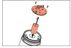
Reverse install LED board and driver by carefully engaging quick disconnects and inserting into fixture body. Secure LED board in place with stainless steel screws. Snap optics in place.
