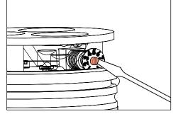
6. With flat head screw driver rotate dial to desired lumen output. Replace cap.
