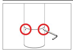
Use a 5/64" allen wrench to slightly loosen three (3) #8-32 stainless steel set screws to remove can
