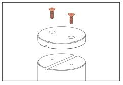
Using a 1/8" allen wrench back out two (2) 10#-24 2. cap screws from clamp to separate.
