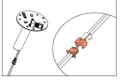
Disengage LED board and driver assembly. Replace with new board and driver assembly.
