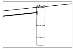
Place connections inside splice compartment. Attach fixture body to splice compartment. Tighten #8-32 stainless steel set screws with 5/64" Allen
