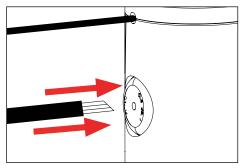
Bring branch circuit wiring with ROUND jacketed line voltage cable to splice compartment. (.130" min to .450" max. dia., Cable By Others)
