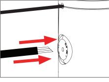
Bring branch circuit wiring with ROUND jacketed line voltage cable to splice compartment (.130" min to .450" max. dia., cable not included).
