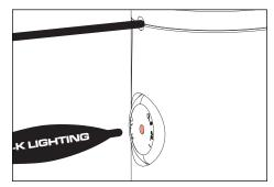
4. Peirce center of Break-Thru Plug with ball point pen
