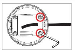
Secure strain relief clamp by tightening two (2) #8-32 3. 2. screws with a 9/64" allen wrench.
