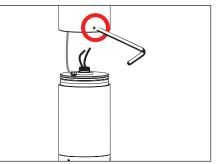
Use a 5/64" allen wrench to separate splice compartment and fixture body.
