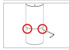
Use a 5/64" allen wrench to slightly loosen 1. three (3) #8-32 stainless steel set screws to remove cap.
