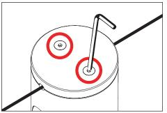
Install clamp to splice compartment to 1/4" O.D. aircraft cable (supplied not included) with two (2) #10-24 cap screws using a 1/8" allen wrench.
