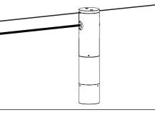
Place connections inside splice compartment. Attach fixture body to splice compartment. Tighten #8-32 stainless steel set screws with a 5/64" allen wrench.
