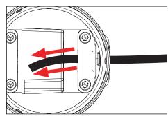
Thread incoming 3 wire ROUND jacketed line voltage 1. cable through grommet, then through strain relief clamp.
