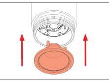
5. Replace optic by lining notches with optic holder, then pressing down gently until secured into place.
