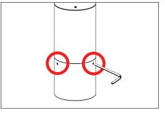
Place 6. cap on fixture and tighten set Tighten screw to 1/2 in-lbs. Top of screws. sit flush screws should with fixture cap.
