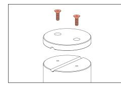
1. Using a 1/8" allen wrench back out two (2) 10#-24 cap 2. screws from clamp to separate.
