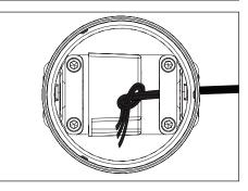
Tie underwriter's knot in cable for additional strain relief between connections and clamp.
