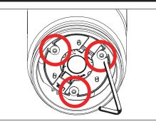
Use a .050" allen wrench to loosen three (3) set screws 3. holding LED assembly. Gently lift LED assembly from fixture.
