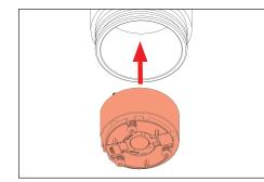
Install new LED assembly. Assembly can only connect 4 in one direction. Secure set screws using a .050" allen wrench.
