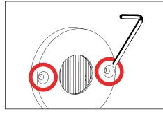
1. Remove fixture by loosening two (2) #10 fasteners. Gently pull from drilled hole enough to expose screw on cap.
