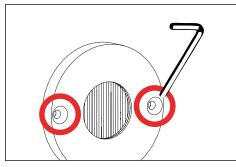
8. Place fixture into core drilled hole, then secure with two (2) #10 fasteners.
