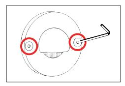
Install fixture into core drilled hole and mount with two (2) #10 fasteners as required (mounting screws supplied not included). Length and type of mounting screws will vary with construction material. Do not over tighten.
