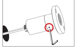
Loosen #8-32 set screw on cap using a 9/64" allen wrench. Remove cap to expose LED board and 2. optics.
