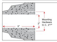
Core drill a 2" dia. hole 5" deep into mounting structure. Select mounting anchors and hardware suitable for building material. Install according to faceplate on-center measurement. Leave sufficient material between core drill hole and anchor mount.
