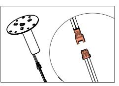
Disengage LED board and driver assembly. Replace 5. with new board and driver assembly.
