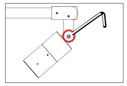
3. Tighten #10-32 stainless steel set screw using a 5/32" allen wrench to secure aiming position.
