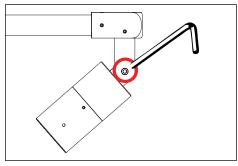
Use a 5/32" allen wrench to slightly loosen #10-32 stainless steel set screw on the stem for 180° aiming purpose.
