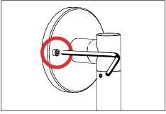
If fixture has larger canopy option, then secure fixture canopy with two (2) #10-24 screws to installed back box using a 1/8" allen wrench. Seal building envelope as per NEC. Do not overtighten.
