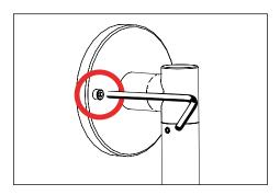
If fixture has standard canopy option, then secure fixture canopy with two (2) #8-32 screws to installed back box using a 9/64" allen wrench. Seal building envelope as per NEC. Do not overtighten.
