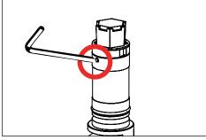
Use a .050" allen wrench to loosen two (2) #4-40 stainless steel set screws below LED board on the heat sink. Gently pull up on LED board and Driver assembly to expose quick disconnect.
