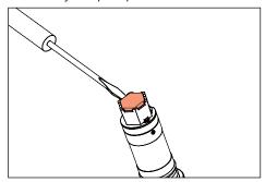
Use small flat head screw driver to remove lens from optic holder on the LED. Snap new optic in place. Replace cap on fixture and tighten set screw.
