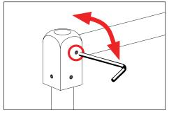
To adjust stem, loosen #8-32 screw with a 5/64" allen wrench at stem cap. Adjust as needed, then secure.
