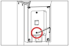
Place connections into bollard. Attach inner bracket with RJ45 jack with two (2) #6-32 screws with a 7/64" allen wrench.
