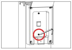
. Loosen two (2) #6-32 screws with a 7/64" allen wrench to remove inner bracket with RJ45 jack.
