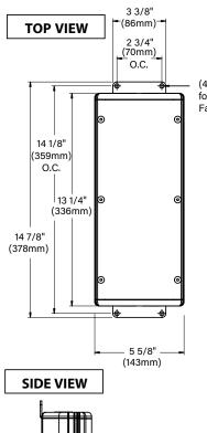
(4) Clearance Holes for 1/4" (6mm) Fasteners (Not Included)
